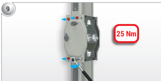
Install the other block joint cover and torque its bolts to 25 Nm.
